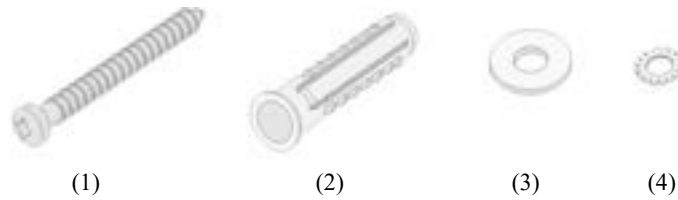
(1) Self-tapping screw M6 (2) Expansion tube (3) Fender washer (4) Spring washer
